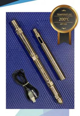
The NeoQ200C Quartz Memory Gauges are developed for extremely high downhole pressure and temperature with sour conditions. The latest innovative hybrid technologies are utilized to greatly extend gauge life into multiple years without replacing the electronic board.
